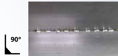
Corner spot welding thickness 0,6 mm
