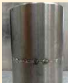
Pipe butt weld Ø 31.75 x 2 mm
