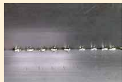
Corner spot welding thickness 0,6 mm
